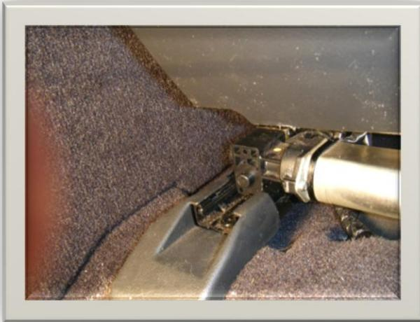
7. Secure the nut on the end of the shaft
