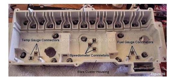
Turn the removed speedometer/odometer panel over being careful to not disturb/damage the speedometer needle. Todd Shrewsbury suggests laying the panel inside the previously removed clear plastic lens to protect the speedometer needle from damage.
