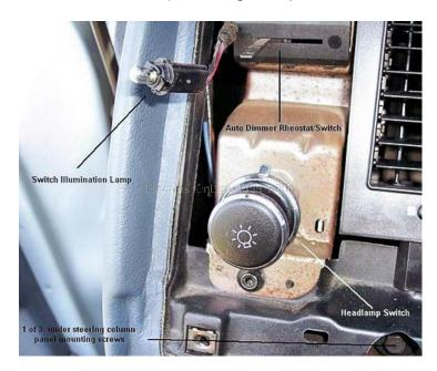
The left and right fascia trim moldings (Pry gently on the outboard ends working towards the center as each clip is pulled free)
