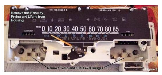
Remove the remaining panel that houses the speedometer and odometers by wedging and lifting as you did the gauges.
