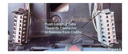
Remove the cluster, being careful to not damage the PRNDL cable. You now have the cluster removed from the vehicle and are ready to find a comfortable chair and a padded table to replace the odometer gears.
