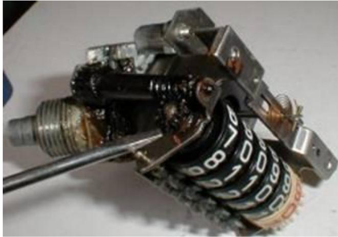
7. **IMPORTANT:** Check the end of the odometer shaft (where the new gear will go) to ensure there are no burrs, bumps or knurling. The shaft must be smooth so as not to crack the new gear. If necessary, use a miniature file smooth the odometer shaft prior to pushing the gear into place.
