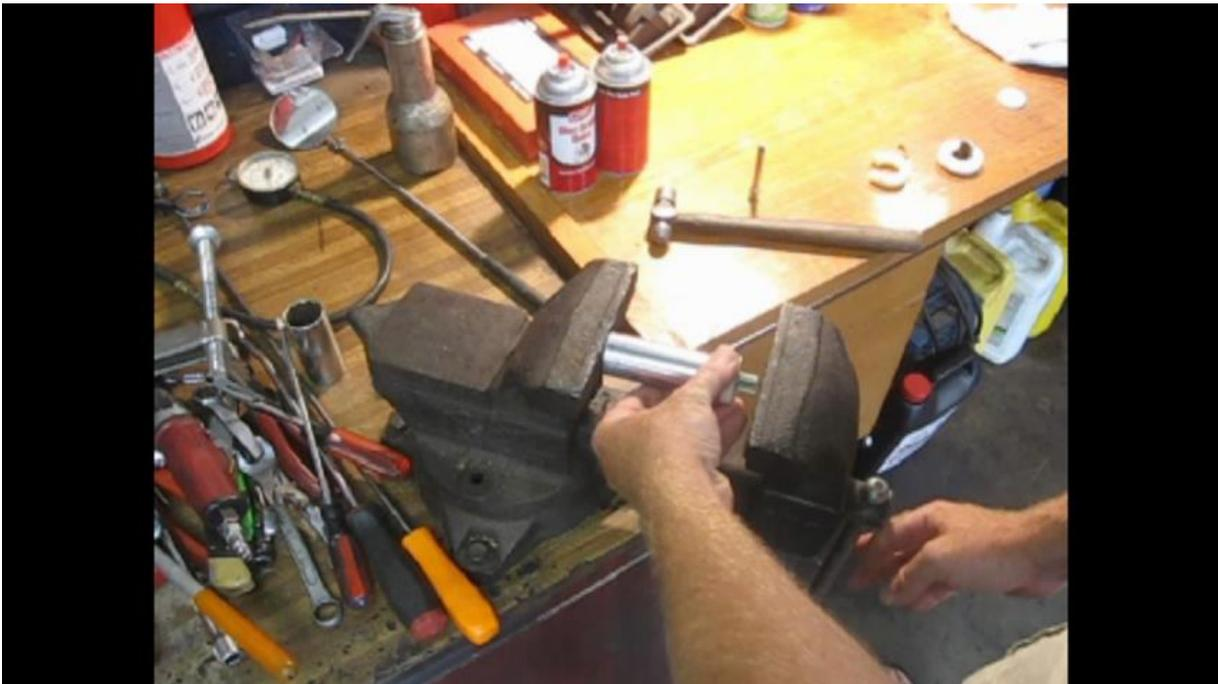
Using a hammer gently tap the metal gear into the new plastic gear until fully seated.
