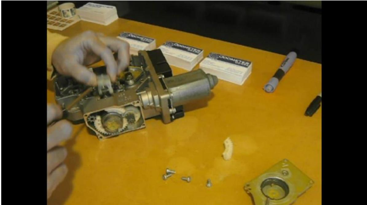
Next unscrew the main shaft that the large gear was on. Also remove the smaller gear, this just pulls straight out.
