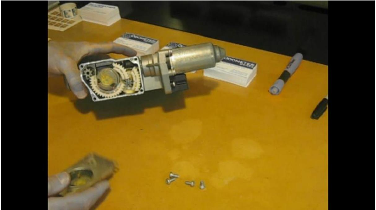
Next remove the T20 Torx screw for the retainer that secures the metal shaft.
