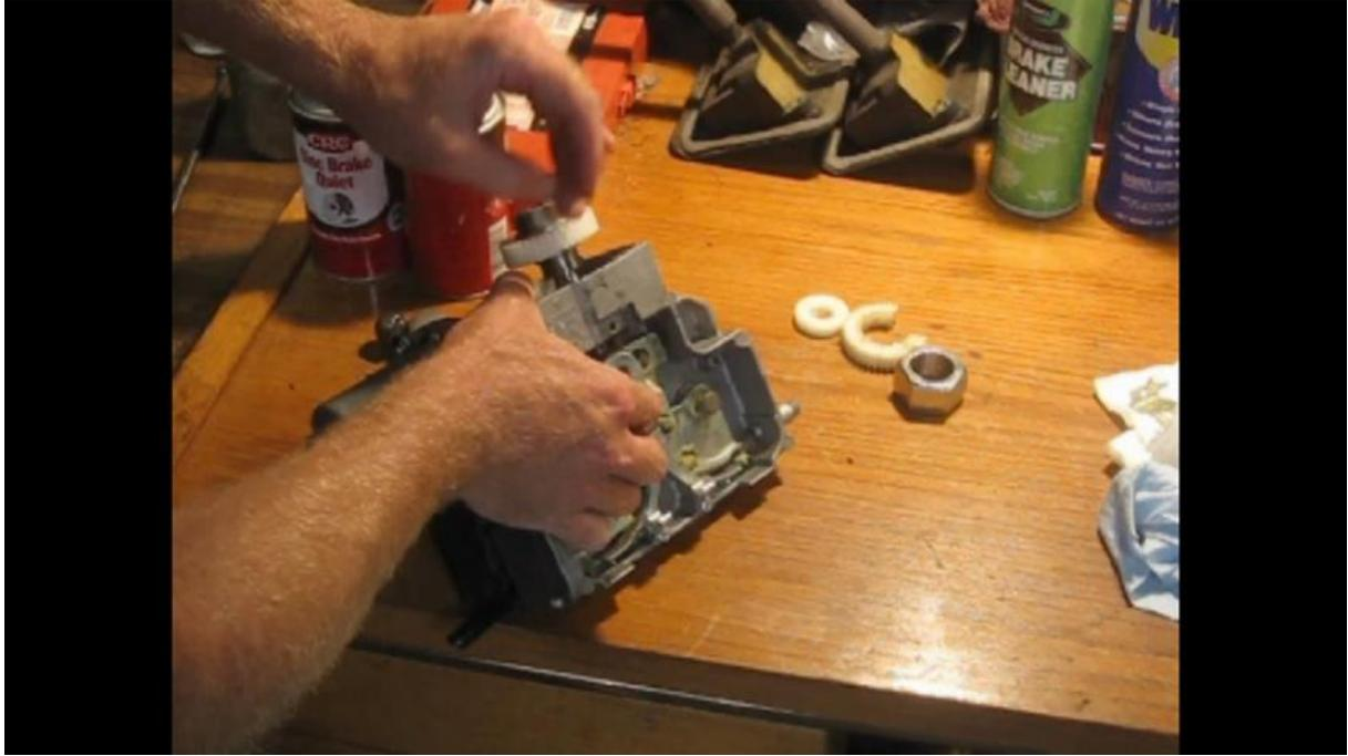
Reinstall the retainer for the shaft with T20 Torx screw.
