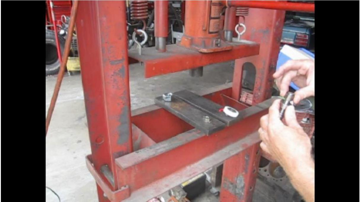
Before installing the new gear apply a small amount of grease to the bushing/bearing section. Press on the upper collar, being careful not to install too tightly as to not bind the movement.
