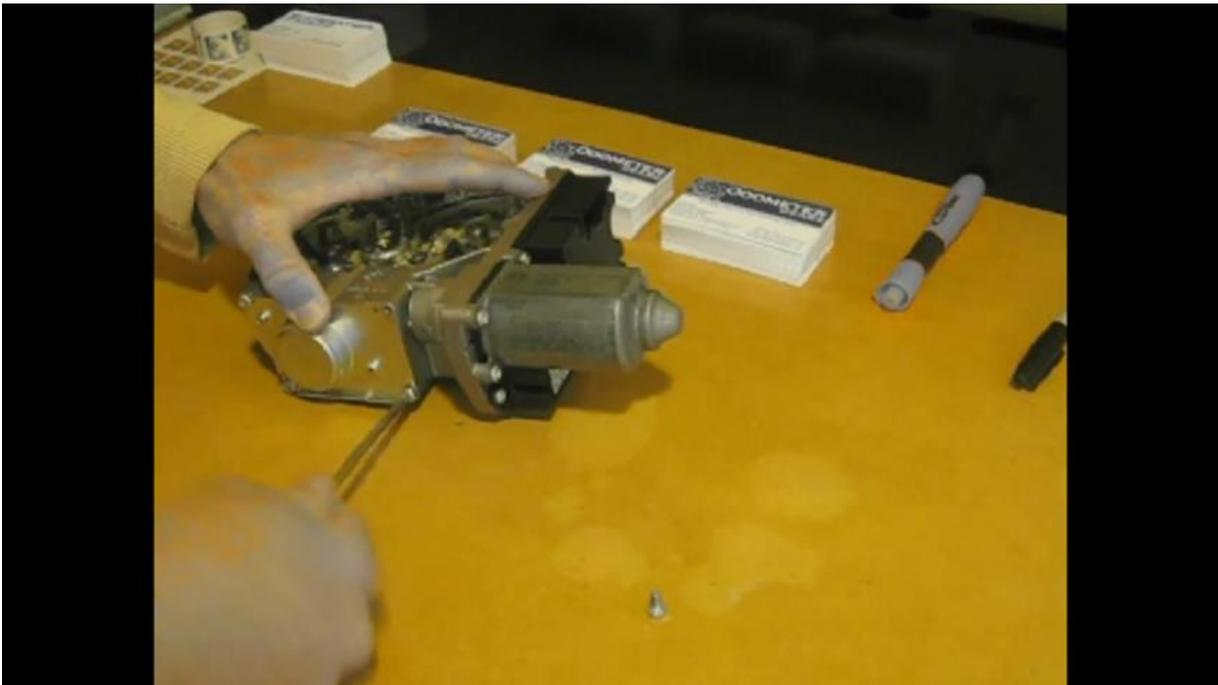
Once you remove the four screws you can remove the cover. Inside you will see the damaged gears.
