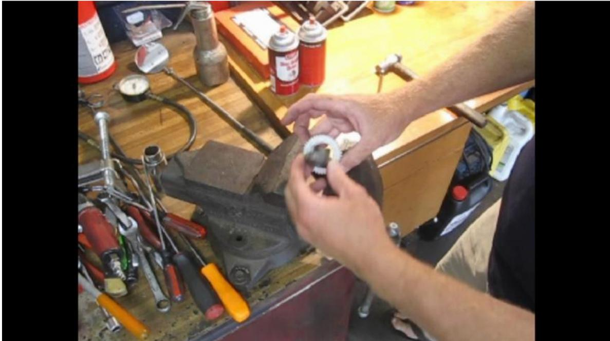
Using a 7/8" socket and a bench vise press the metal gear out of the plastic gear.
