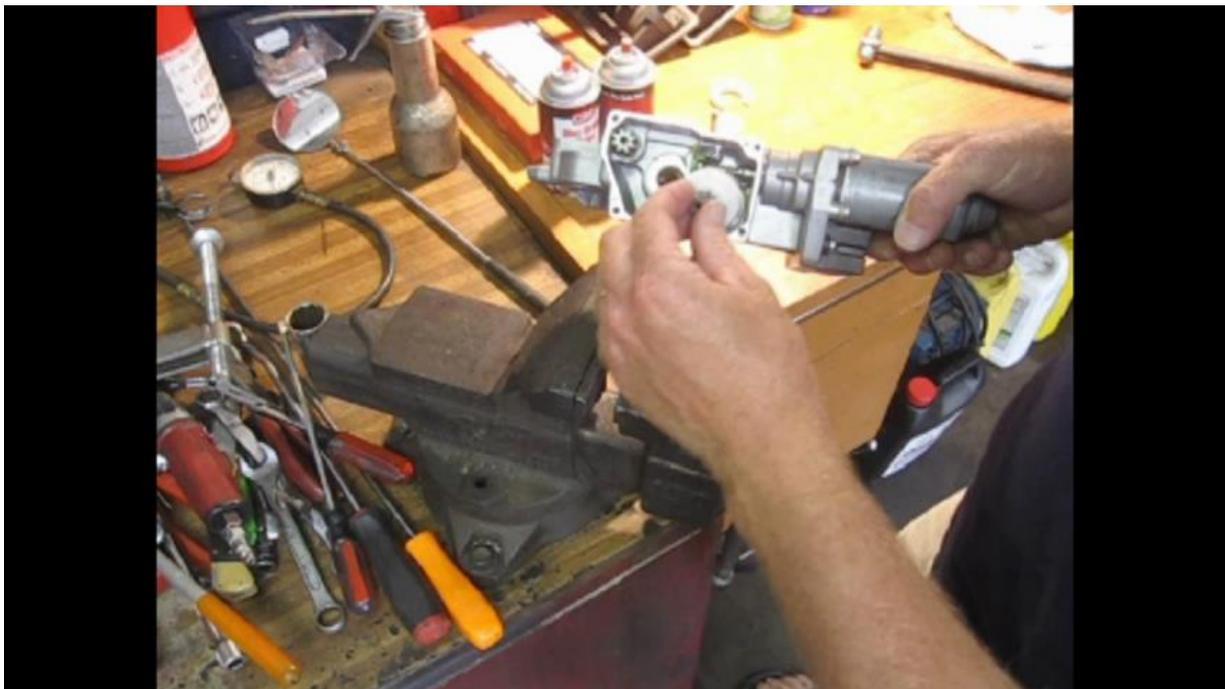
Now press together the parts on the larger shaft in the reverse order removed. Make sure to fully seat each part.
