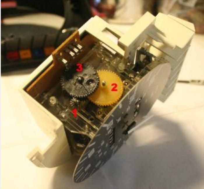
Go ahead and remove the two shafts and the attached gears, and clean them down to remove the excess grease. In the image below, I have one shaft still installed along with gear 5 which we keep from the original set. You also see gear 1, which we're going to remove. Try to pull it off, it's pretty much going to turn to mush and fall to pieces, leaving a bronze insert stuck to the shaft.
