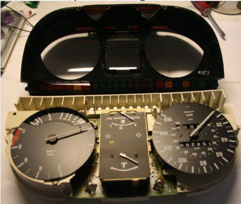
Next, you'll need to split the speedometer portion of the cluster out so you can access the gears. With the needles facing upwards, like in the picture below, you'll have to push out the speedo section. You do this by pushing it out of the cluster from the back. There is going to be some resistance as you're disconnecting a 5-pin connector as you do this. The connector is shown below - you'll want to push on the back of the cluster in the vicinity of this connector.
