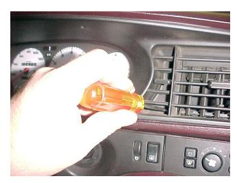
8. Lift up on the bottom edge of the trim piece right behind the steering column trim piece. This will allow the gauge cluster trim top of the steering column. You may also need to pull down slightly on the top of the trim piece to clear the dash. The instrument cluster trim piece should now slide out of the dash.
