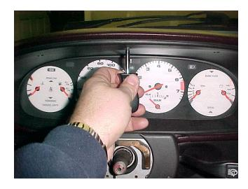
6. Remove the two Phillips head screws which thread into the plastic trim piece from the bottom on either side of the steering column.
