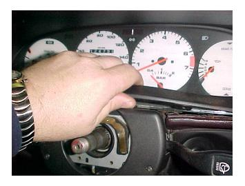
9. With the trim piece removed, you will now see the four Phillips head screws which hold the gauge cluster in the dash. Remove the screws and slide the cluster forward to access the electrical connectors on the back of the cluster.
