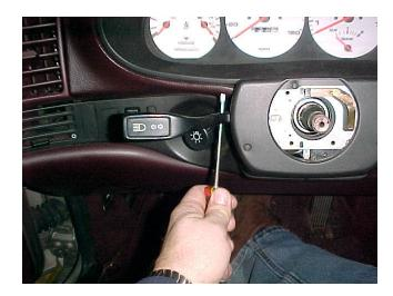
7. The vents in the center of the dash are an integral part of the trim piece surrounding the instrument cluster. There are several Phillips screws located in the vents which must be removed to remove the instrument cluster trim piece. There is one Phillips head screw located in the vent
