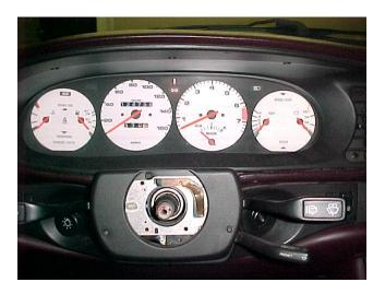
5. Remove the three Phillips head screws located in the top of the plastic trim piece around the gauge cluster. A stubby Phillips head screwdriver works well here.
