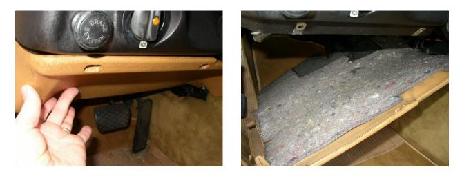
Remove the hush panel under the driver's side dash. There are 3 Phillips screws on the top and 2 plastic Phillips half turn locks, 1 on each lower side.
