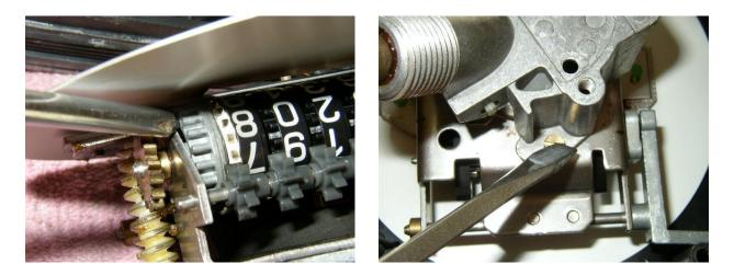
Ahhh we found the problem! The pot metal gear that the screwdriver is pointing to should NOT be turnable without the entire shaft and numbers advancing. This gear in fact does "slip" on the shaft, hence the numbers
