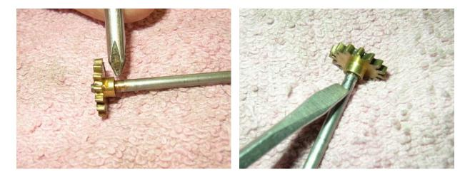
With the shaft removed you can see the shinny spot where the pot metal gear was slipping and spinning.
