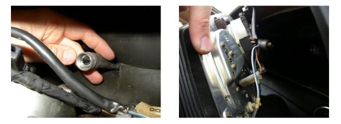
Disconnect the Speedo cable and remove the clock connection, the seat belt and glow plug connections, Speedo electrical connection, and tach connection.
