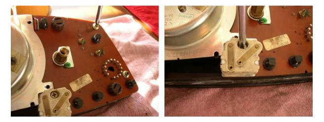
Remove the 2 screws holding the gauge cluster and the dimmer switch. If your dimmer switch does not work, now would be a great time to replace it.
