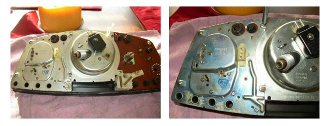
Take the cluster and put on a clean towel in an area with good lighting. Then remove the 4 screws holding the clock cluster.
