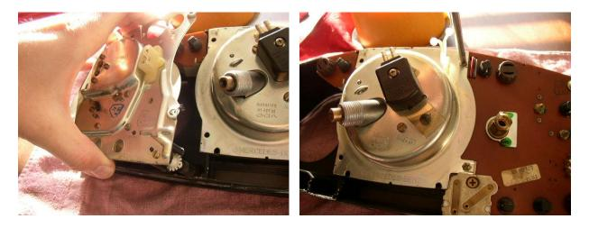
Gently lift out the clock cluster and set aside. Remove the 2 screws holding the Speedo to the cluster, but do not remove just yet.
