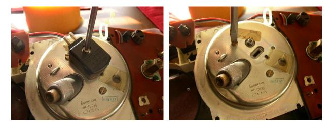
Remove the Speedo electrical box. Then the 2 screws holding the rear of the Speedo.
