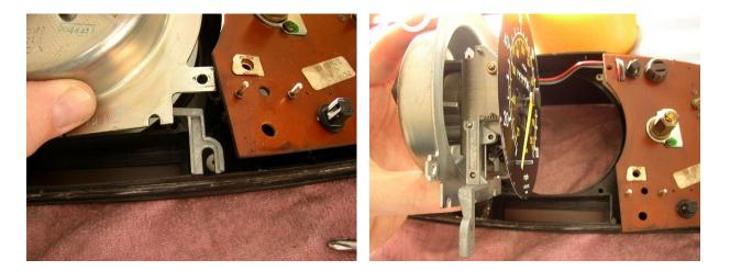
Gently lift the edge of the gauge cluster closest to the Speedo. Lift out the Speedo and pay close attention to the trip meter reset arm, which is why we lifted up the gauge cluster. This makes it much easier to get the Speedo in and out of the cluster without damaging the reset arm.
