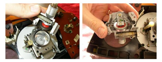
Lift straight up and be careful to grab the vertical plastic gear and set aside. Seen in next pic.
