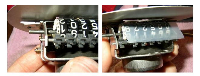
This is by far the hardest part! Putting the geared shaft back into the number set and getting the pot metal gear back into position. It took me about 1 hour to do it. There is very little clearance and the shaft obviously must be out at the point where the gear is slid back in. This causes the other numbers to move and often fall out.
