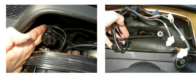
Disconnect the master harness for the gauge cluster. It is usually quite tight so just pull gently straight out, don't rock it side to side. This is the whole harness for the cluster.
