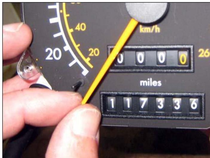
Grip the needle at the center pivot point and rotate counter clockwise, you will feel some resistance as you turn the needle. **DO NOT PRY UP OR PULL UP ON THE NEEDLE!** This is normal as you are using the internal stop to help remove the needle. It is like you are unscrewing the needle and it will start to feel loose the more you twist the needle. You will get to a point that it feels very loose and at this point give the needle a very slight pinch and this will release the needle.
