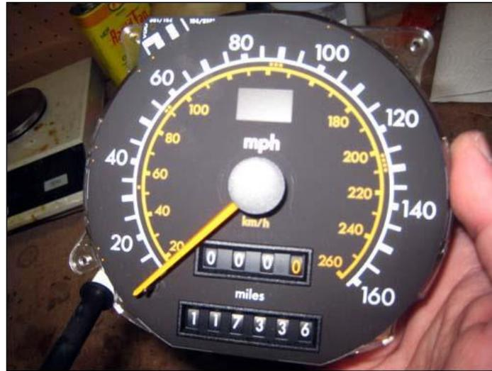
Carefully raise the tip of the needle over top of the needle stop. Place a mark where the needle points on the very edge of the face of the speedometer and this is where you will need to line the needle back to after the repair is completed.
