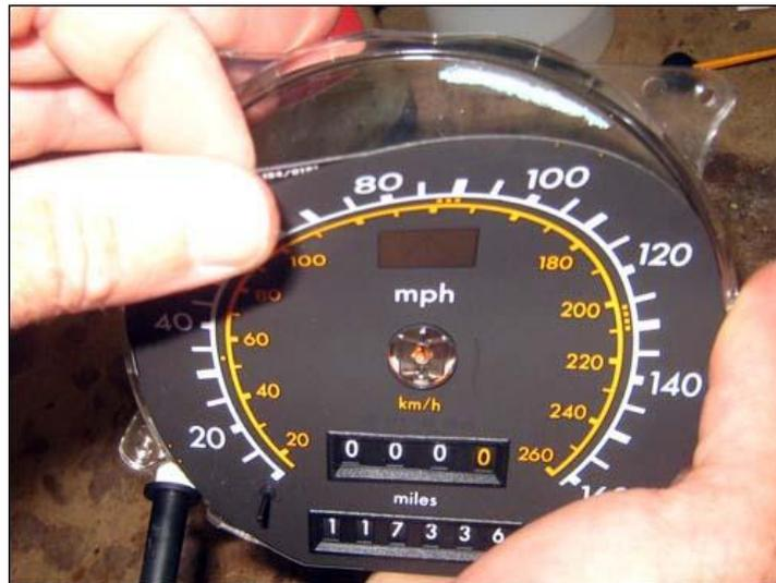
Once the face plate is mostly removed you will need to remove the needle stop. Place your fingers behind the numbered face plate around the needle stop. Apply upward pressure with one hand and you use the other hand to twist and pull out the stop. The plastic trim rings around the odometer and trip meter will pop out the same way.
