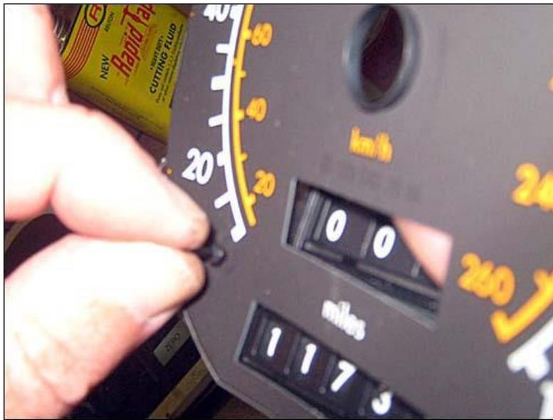
Once the stop is removed you can remove the face plate. Be sure to place the face, face down on a soft surface. You will not need to use an additional adhesive to reinstall the face as long as you do not damage the glue. Use a small standard screw driver and remove the two screws that hold the face plate housing to the motor housing.
