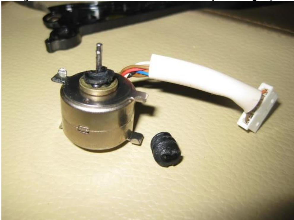
**Once the motor is removed you will see the worm gear attached to the bottom side of the motor. Remove the old worm gear by pulling it off with your fingers or a flat blade screw driver. Install the new worm gear using channel lock pliers or a bench vise leaving the thickness of two business cards between the motor and the gear. The new gear is installed with the neck towards the motor housing.**
