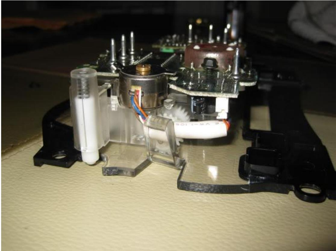
On each side of the motor here you can see the clear plastic clip that holds it in. The motor has tabs on it that when you twist it, go under the plastic tabs. So to get the motor out, you have to push down on it and twist to get it out.
