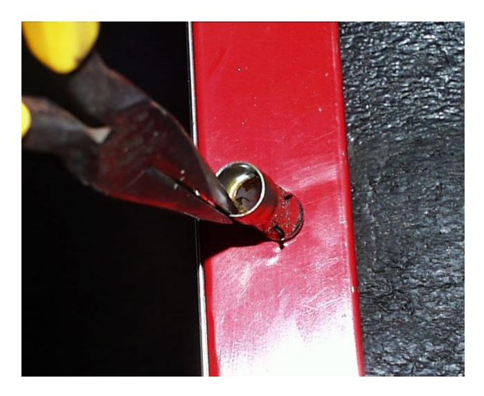
Sometimes there is a hard plastic thing or a blob of grease or a rubbery piece of snot or fuzzy thing or nothing that lives in this space. Give the end a 3-4 second shot with the torch and stab it back on to the mark Now stick the drive cable back into the sheath you may need to twist and jiggle to reengage the other end. If you are worried about overheating the end have a wet towel ready to slap on it.
