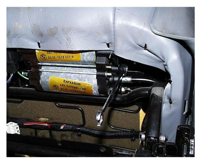
Take the bolts out of one end at a time. Once the bolts are out tip the motor out and pull the cable out (memory seat note, on one end of each motor is a
