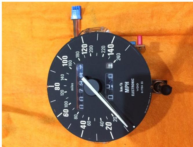
Next you need to peel the face off the plastic housing to access the screws that secure the front and rear halves of the speedometer. The gauge face is held on with sticky contact glue. Be careful and peel the gauge face from the plastic housing and place face down on a clean surface. You do not need to apply any additional glue when you reinstall the gauge face. Now remove the screws that secure the plastic cover to the back of the speedometer.
