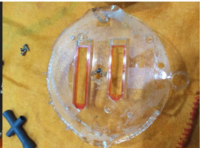
Now that the face is removed you can access the two screws that hold on the stepper motor circuit board to gain access to the odometer gear and pod.
