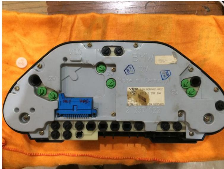
Remove eleven (11) screws that secure the grey plastic backing
