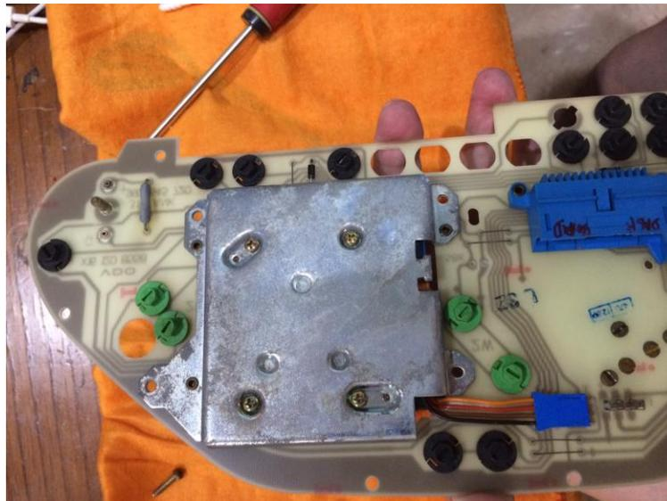
With the speedometer out of the cluster the next step is to remove the speedometer needle. Before beginning make a small mark on the very edge of the speedometer face where the needle is pointing as this is where the needle needs to line up when the job is complete. Sometimes there is a factory mark but your needle may rest slightly higher or lower. This will help to ensure the speedometer is close to the proper speed calibration when driving.
