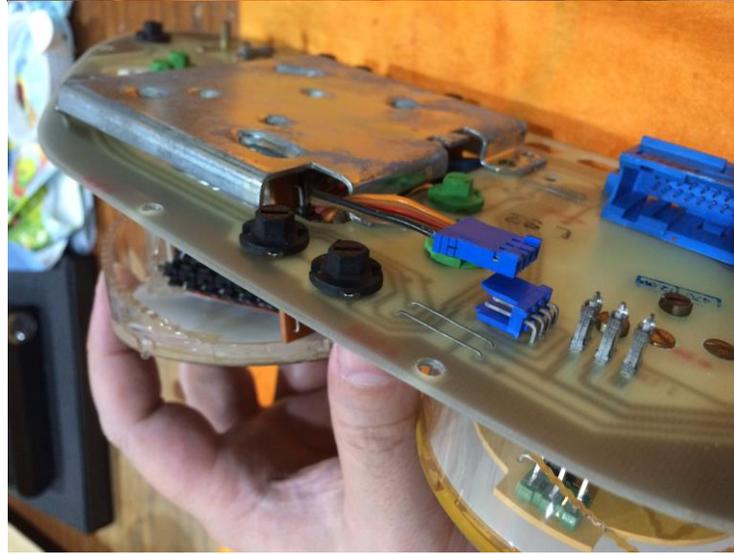
Remove four screws that secure speedometer into cluster.
