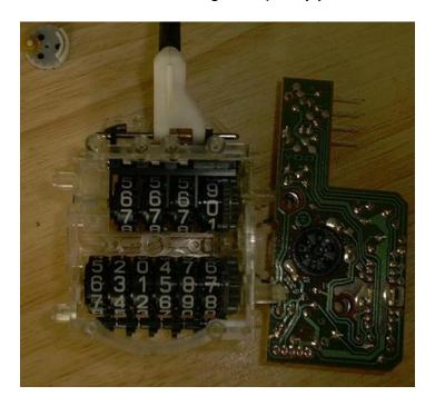
The next picture is a close-up of the odometer gears for the odometer motor. The yellow gear will fall off the white plate so be careful not to lose it. The small yellow gear is the most common to fail. The white plastic disc has a gear on the bottom side and will also fail as it is made from the same material. Both the gear and the pod are available from OdometerGears.com
