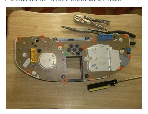
Once these screws are removed the cluster circuit board will be free. You can carefully pull the circuit board off and get ready to dig into the speedometer. If you were having problems with both the odometer AND the speedometer than this is likely as far as you'll need to go. Step six: Now that you have the speedometer, you need to disassemble it. The first step is to remove the speedometer needle.
