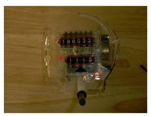
Step eight: Next, remove the odometer screws. Flip the odometer on its side and removed the screws circled below.
