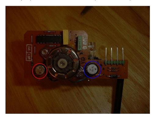
Each capacitor above has two pins that go through to the other side. On each capacitor, locate and test these two pins for continuity (ohms). You should read infinite ohms (open circuit). The one circled in blue was shorted on my car. Shorting of this capacitor created a short between the positive and negative connections to the speedometer motor. Hence, my speedometer guit working.
