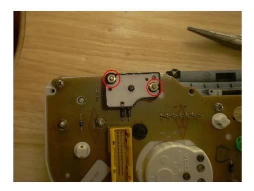
Then pull the rheostat straight out. *Step four:* Now the screws that hold the back of speedometer need to be removed. The following picture indicates the speedometer screws in orange. Automatic cars or B4's equipped with an outside temperature display will have an electrical connector that needs to have its screws removed where the blue circles are located.
