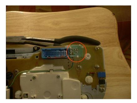
Next, pull the wire away from the cluster so the circuit is not restrained. Then pull the auto-check system straight out. *Step three:* The next step is to remove the rheostat. This is done by removing the nuts circled below.
