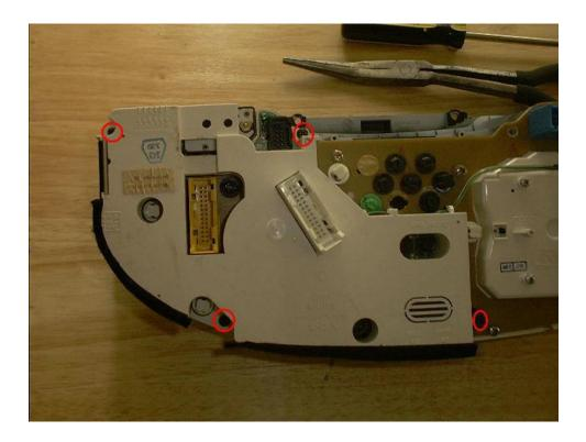
Once the screws are removed you need to disconnect a small circuit that runs across the cluster. This circuit just simply unclips and is shown below.
