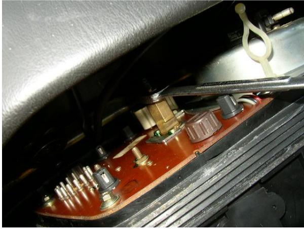
**This is why you want some slack on the Speedo cable. The cluster can move forward allowing you to get your hand behind. Remove the oil supply to the gauge with a 10mm wrench.**
