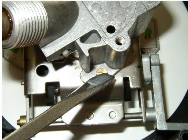
Ahhh we found the problem! The pot metal gear that the screwdriver is pointing to should NOT be turnable without the entire shaft and numbers advancing. This gear in fact does "slip" on the shaft, hence the numbers
