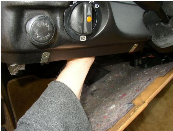
**Reach under the dash and gently pull the odometer cable an inch or 2 through the firewall. This will give you a little more room to get your hand behind the dash cluster when you loosen the cluster.**
