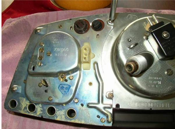
**Take the cluster and put on a clean towel in an area with good lighting. Then remove the 4 screws holding the clock cluster.**
