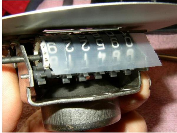
**This is by far the hardest part! Putting the geared shaft back into the number set and getting the pot metal gear back into position. It took me about 1 hour to do it. There is very little clearance and the shaft obviously must be out at the point where the gear is slid back in. This causes the other numbers to move and often fall out.**
