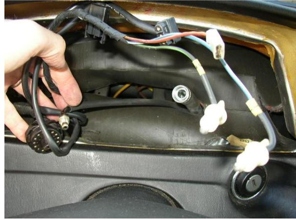
**Disconnect the master harness for the gauge cluster. It is usually quite tight so just pull gently straight out, don't rock it side to side. This is the whole harness for the cluster.**
