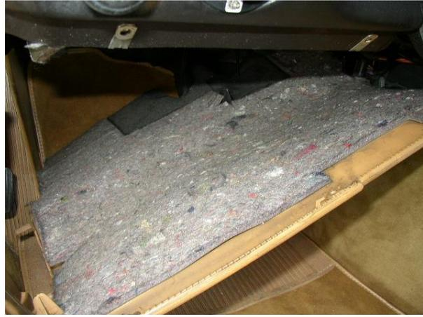
**Remove the hush panel under the driver's side dash. There are 3 Phillips screws on the top and 2 plastic Phillips half turn locks, 1 on each lower side.**
