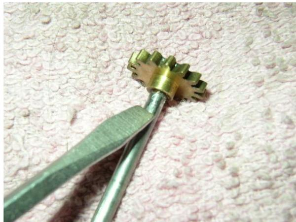
**With the shaft removed you can see the shinny spot where the pot metal gear was slipping and spinning.**
