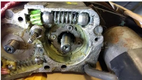
**!!!NOTE: If you remove the large gear there is a plastic thrust washer that is generally stuck to the bottom of the gear with grease. Remove the washer and align with the four screw heads inside of the housing. Reinstall the gear. If you do not have the washer aligned properly you will not be able to secure the cover as it will not sit flush!!!**
