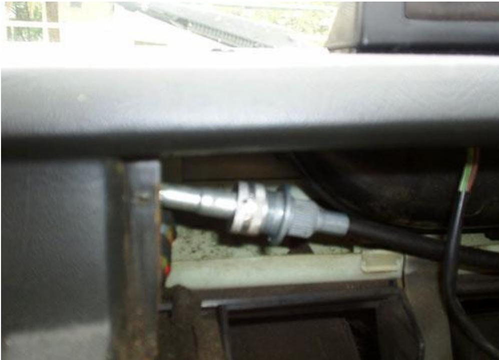
Unscrew the speedometer cable. The connection is underneath the air vent in the centre of the dash. Simply unscrew the cables and pull apart.
